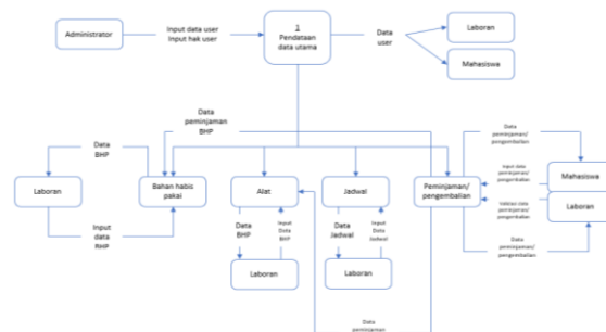
Gambar 2. Diagram Level 0 Sistem Inventaris LabKu
